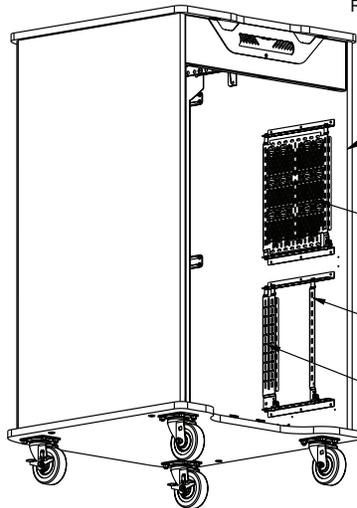
LEFT RACK SIDE CAN MOUNT (2) LEVERLOCK ADAPTERS FOR RFR-2428XX AND RFR-2028XX, AND (1) ADAPTER FOR RFR-1628XX
